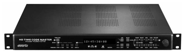
The HD9010TM HDTV Time Code Master is a full function time code reader/generator system for high definition serial digital video. The HD9010TM is a combination dual generator/dual reader for Linear Time Code (LTC) and SMPTE 12M-2 Ancillary Time Code (ATC), and contains a high resolution character inserter which can burn the generator or reader numbers directly into the serial digital program output.
